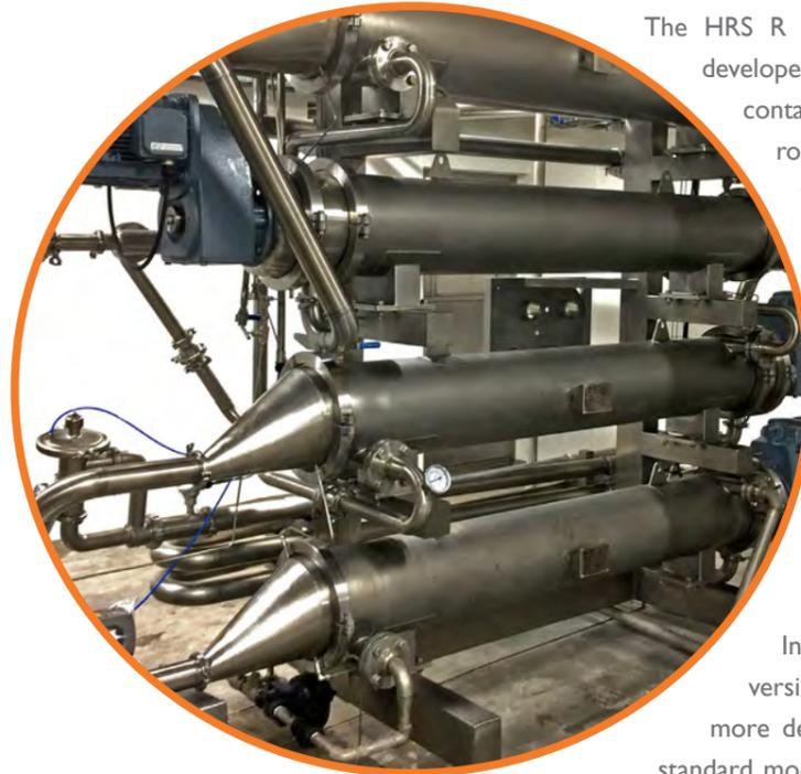
The HRS R Series is a rotary scraped surface heat exchanger developed for hygienic applications. Each inner tube contains a scraper bar fitted with a helical screw which rotates at high speed and enhances flow through the tube whilst reducing pressure drop. Furthermore, the continuous scraping action eliminates fouling on the inner tube wall, ensuring that the heat transfer area is clean at all times.
